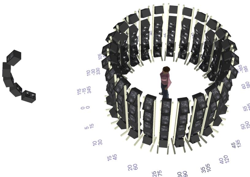
Right hand side: the actual speaker setup that is the result of the audio ease sampling procedure, and left hand side: a single vertical stack artificially extended to place the speakers on a sphere. The speaker setup used in the 360monitor in 9 channel mode has been picked from these positions.
