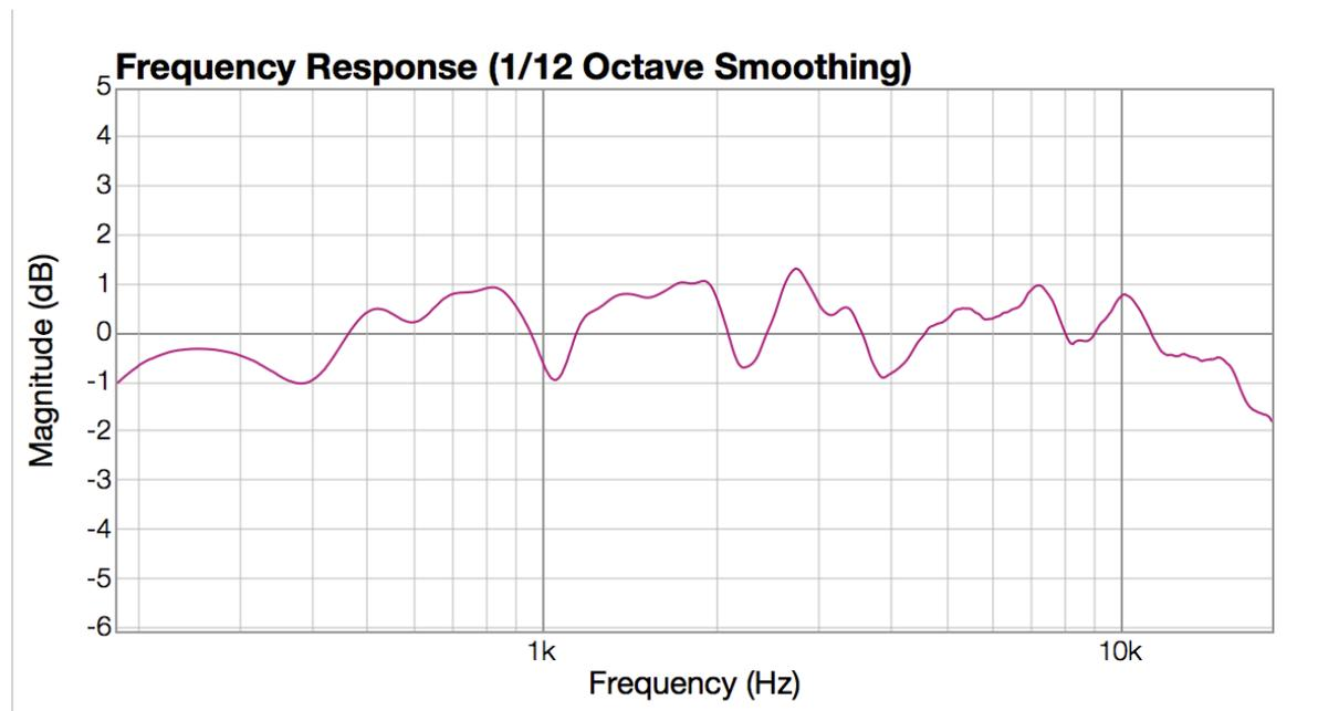
Magnitudes per frequency of an Impulse Response of length 480 samples (10 msec) taken from a Genelec 1031 to a Knowles miniature omnidirectional microphone in the Audio Ease anechoic chamber. It stays within 3 dB throughout the frequency band that ends up in the final IR.
