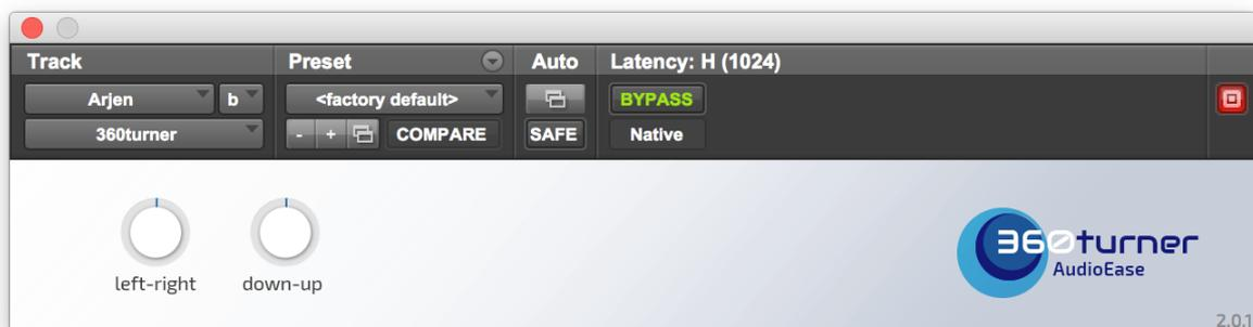
The 360turner together with 360radar allows you to rotate or tilt an ambisonics recording so that misalignment and calibration errors of the microphone can be easily corrected.
