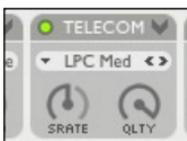
By applying actual telecommunication industry standard audio data compression such as 'GSM', this module faithfully reproduces the typical audio artifacts found in bad phone connections. Repetitions, underwater effects, it will all sound very familiar. As a side effect of the LPC coder/decoder the Telecom module doubles as a classic
