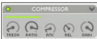
**The horizontal meter** - continually displays the amount of gain reduction. The dynamics section is completed by the limiter near the 'OUT' control at the right top.
