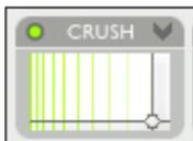
Drag the cross hair down to reduce word length (reduce from 32 bit input to 2 bit output). Move to the left to reduce sampling rate. To maximize aliasing effects the most crude of sample rate conversion algorithms lies beneath the Crush module.
