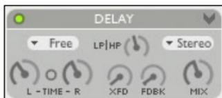
**STEREO MONO** - in mono mode the delay output is summed to mono
