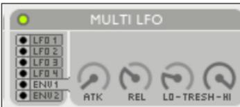
Connecting is done similar to an LFO. An envelope follower increases the value of the connected parameter according to the level of incoming audio. It starts reacting when audio exceeds the lo-threshold, and it will not increase further when the level exceeds hi-threshold. Attack and release determine how quick the envelope follower reacts.
