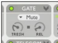
**TRESH** - Threshold - the gate mutes or attenuates the signal when it drops below this threshold level.
