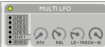
Connecting is done similar to an LFO. An envelope follower increases the value of the connected parameter according to the level of incoming audio. It starts reacting when audio exceeds the lo-threshold, and it will not increase further when the level
