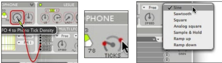
(left) LFO 4 gets connected to parameter Gramophone Ticks (centre) minimum and maximum of Ticks are set. LFO 4 will swing it between these values. (right) shape and speed of LFO 4 are set in the LFO module.
