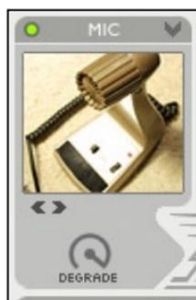
Similar to the speaker selector, but here a microphone impulse response can be selected. The available microphone impulse responses capture time and frequency characteristics of the microphones depicted, and therefore make it sound as if the selected microphone was used in the result. Use it to make an announcer speak through a typical announcer microphone, or to pick up a guitar cabinet using a classic microphone for the purpose, for instance a Royer.
