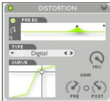
In the distortion module audio is first passed through the Pre EQ. If you engage it by clicking its on/off button you can control both a parametric EQ and a low pass filter with resonance in the same graph. Bandwidth, or Q, for the Parametric EQ can be adjusted with the small rotary control.
