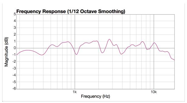
Magnitudes per frequency of an Impulse Response of length 480 samples (10 msec) taken from a Genelec 1031 to a Knowles miniature omnidirectional microphone in the Audio Ease anechoic chamber. It stays within 3 dB throughout the frequency band that ends up in the final IR.
