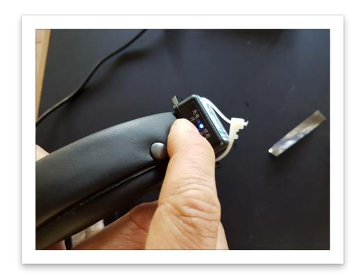
Switch the device on by sliding the knob to the left (a blinking blue light should appear, if not revert to 'charging the head tracker').
