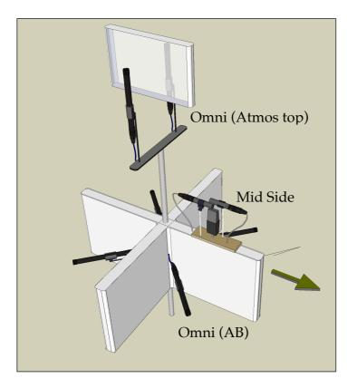
All Impulse responses have been recorded using the same nine-microphone rig. There are two quad surround systems, one comprised of four DPA 4006 omnidirectional microphones spaced by baffles. We (wrongly) call this the AB system.
